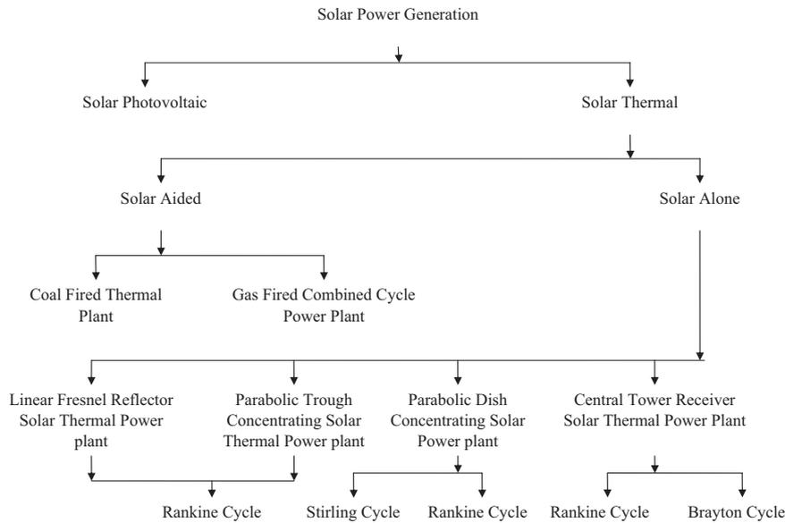
Fig. 1. Schematic view of solar power generation methods.
