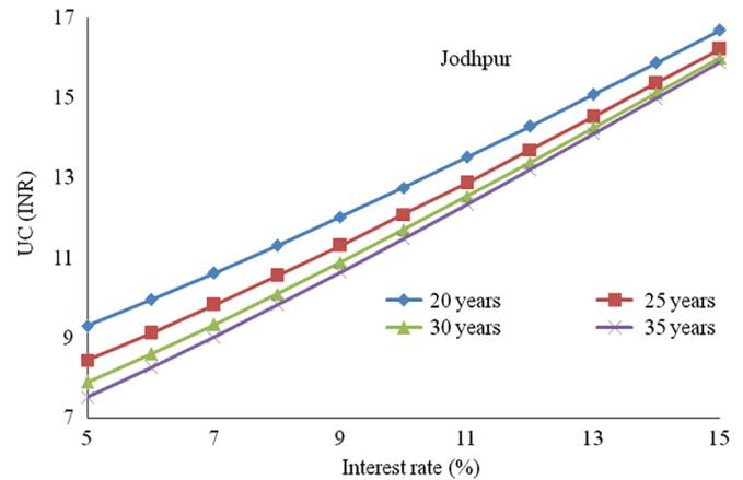
Fig.3. Variation of unit (kWh<sub>e</sub>) electric energy generation cost (UC) with interest rate (%) of PTCSTPP for the Jodhpur location [123].
