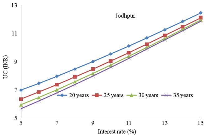
**Fig. 6.** Variation of unit (kWh<sub>e</sub>) electric energy generation cost (UC) with interest rate (%) of PDCSSPP for the Jodhpur location [120].
