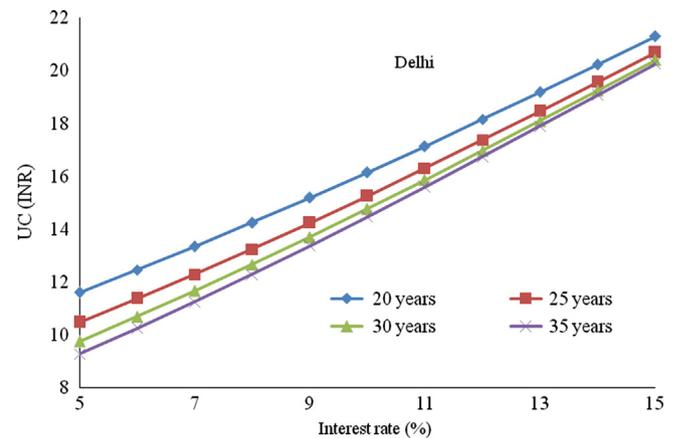
Fig. 4. Variation of unit (kWh<sub>e</sub>) electric energy generation cost (UC) with interest rate (%) of PTCSTPP for the Delhi location [123].
