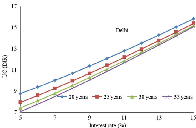
**Fig. 7.** Variation of unit (kWh<sub>e</sub>) electric energy generation cost (UC) with interest rate (%) of PDCSSPP for the Delhi location [123].
