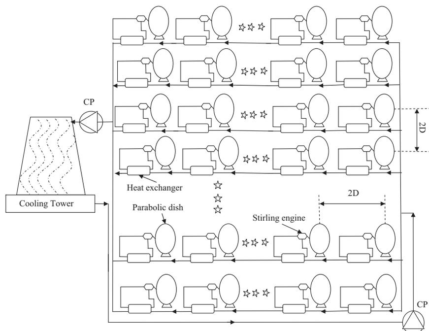
Fig. 5. Simplified schematic view of the 50 MW<sub>e</sub> parabolic dish concentrating solar Stirling engine power plant [120].
