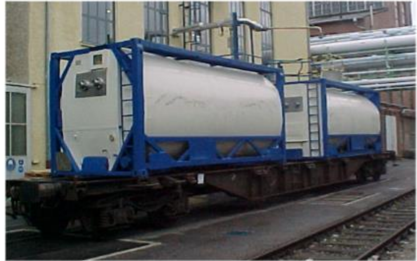
Figure 22: Railway wagon with a latent heat storage system (Source: TransHeat GmbH)
