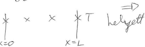
$$\left. \begin{aligned} \rho c_v \frac{\partial T}{\partial t} + \nabla \cdot \underline{q} &= 0 \\ \tau_q \frac{\partial \underline{q}}{\partial t} + \underline{q} &= -\lambda \nabla T \end{aligned} \right\}$$
